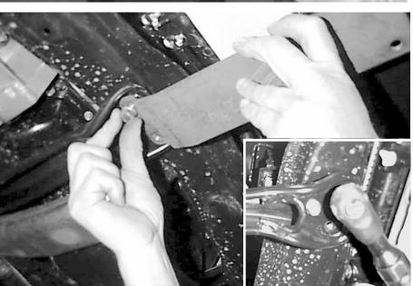
4. Install center support brace by taking two bolts out of vehicles center brace. (NOTE: Be sure to leave in the third bolt, only remove two bolts.) Attach center support to vehicle using two 10mm x 1.25 x 30mm bolts and 10mm lockwashers. Snug tighten these bolts and secure front of support using two 3/8" x 1-1/4" hex bolts, lockwashers, flatwashers and hex nuts. Push cross member up and tighten all bolts.
